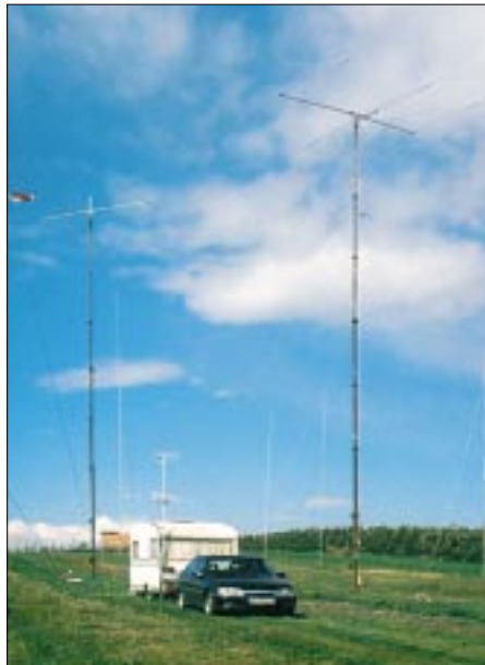
Antennenpark von DK0VD/p (10-m-4-Element-Yagi, FB3, 80-m-Groundplane, 40-m-Groundplane 2-Element-Array, 80-m-Delta Loop, 40-m-Delta Loop, 160-m-Dipol)
